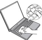
3 Slowly lift up the computer, keeping it level, and wipe any water coming out of the holes on the bottom using a soft, dry
