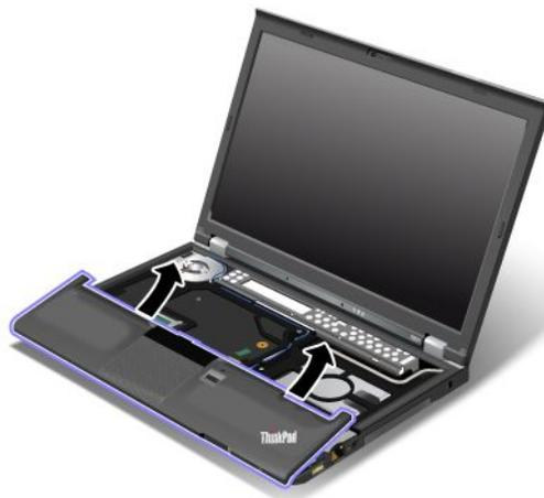
9. Release the palm rest from the computer. Now the palm rest has been removed.
