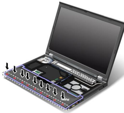
3. Attach the flip-lock ZIF connector **1**, then push the palm rest cable **2**.
