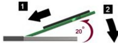
**Note:** If you install a memory module in only one of the two memory slots, install it in the lower slot.
