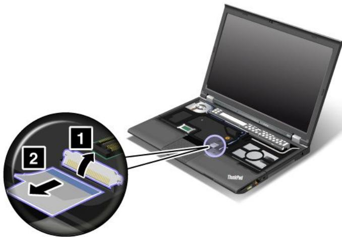
8. Lift up and remove the palm rest.
