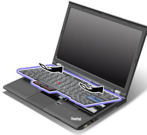
3. Press gently on the areas marked in the drawing, and slide the keyboard toward you. Make sure that the edges of the keyboard marked in the drawing, are under the frame.
