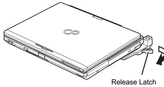
Figure 47. Unlatching the Port Replicator
