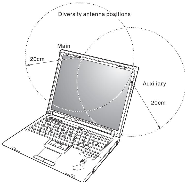
**Note:** The transmission diversity function is implemented for the cards. The function does not emit radio frequencies simultaneously from both antennas. One of the antennas is selected automatically or manually (by users) to have good quality of radiocommunication.
