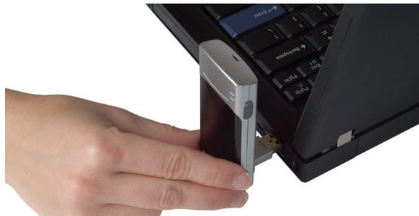
Figure 3-3: Correct way to insert the AirCard USB modem
