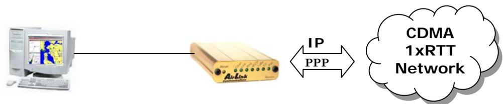
If the host establishes a PPP link to the AirLink modem, a second PPP link is created between the modem and the host. IP packets can then be sent to and received from the 1xRTT network.
