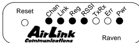
Note that the **RSSI** light may be flashing or solid, showing the strength of the signal. Also the **Tx** (transmit) and **Rx** (receive) lights will flash as data is transferred to and from the modem on the network.
