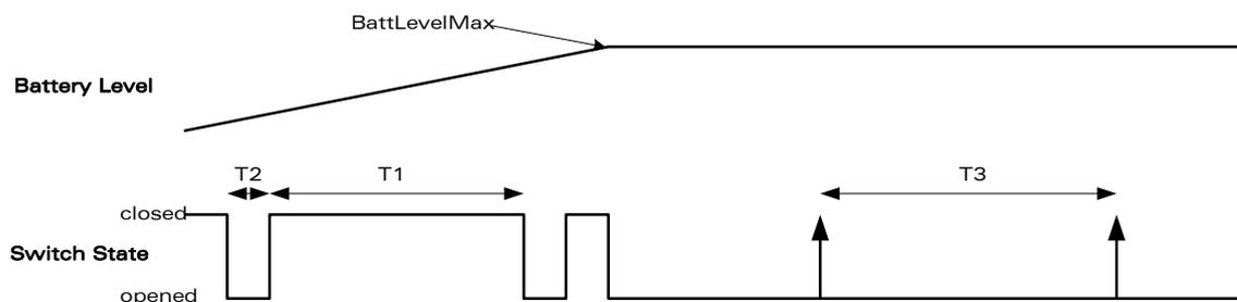
Figure 7: Ni-Cd / Ni-Mh charging waveform
