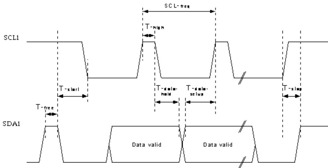
**Figure 6: I<sup>2</sup>C Timing diagrams, Master**
