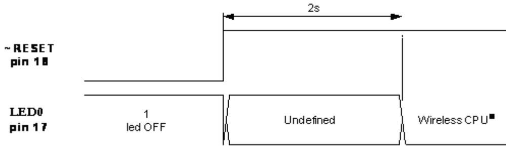
**Figure 13: LED0 state during RESET and Initialization time**
