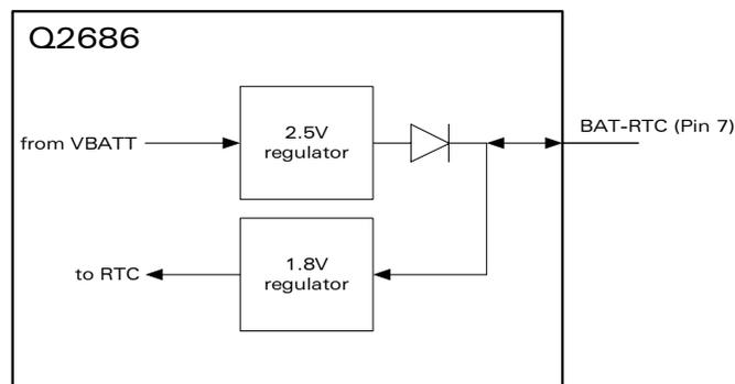
Figure 12: Real Time Clock power supply
