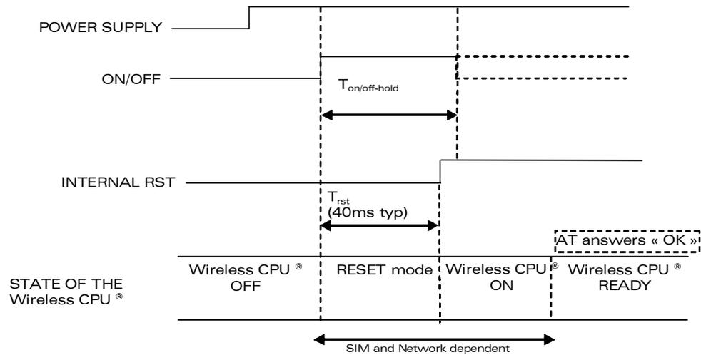
**Figure 9: Power-ON sequence (no PIN code activated)**
