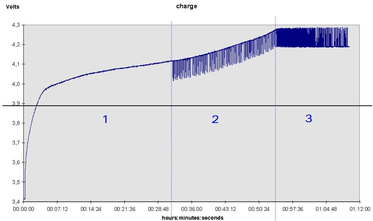
Figure 8: Li-Ion full charging waveform
