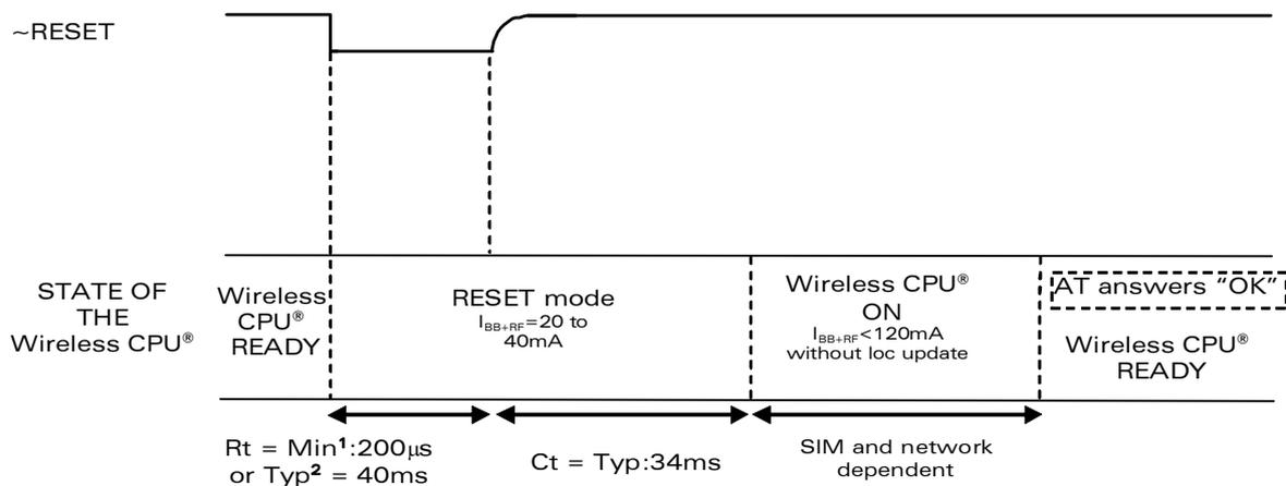
**Figure 11: Reset sequence waveform**
