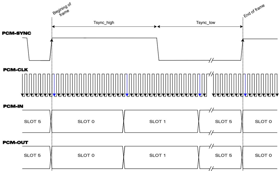
Figure 14: PCM frame waveform
