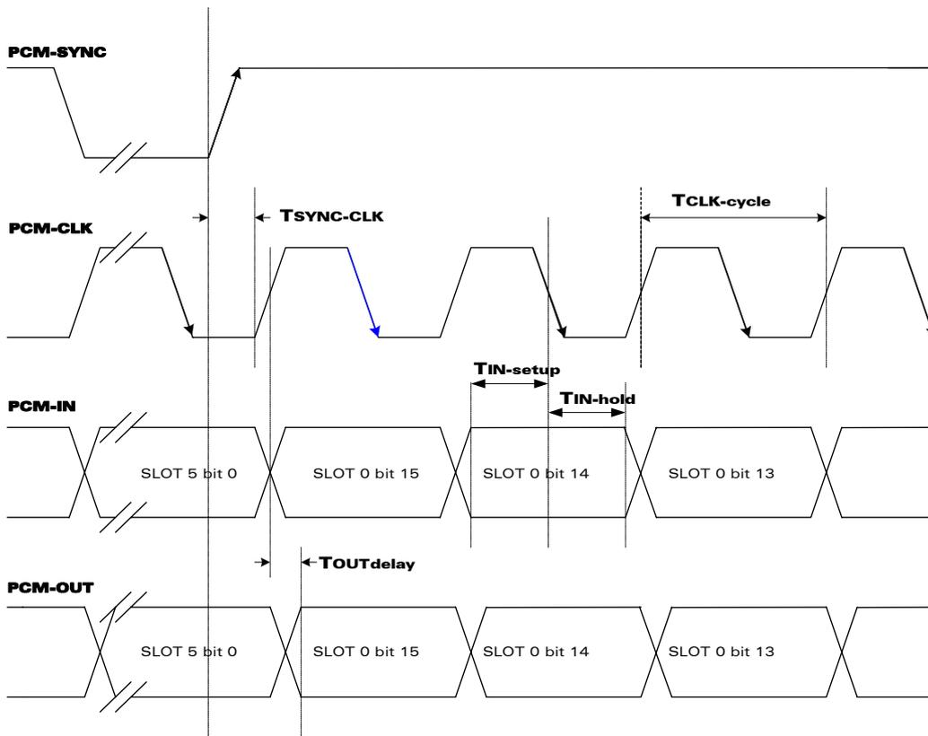
Figure 15: PCM sampling waveform
