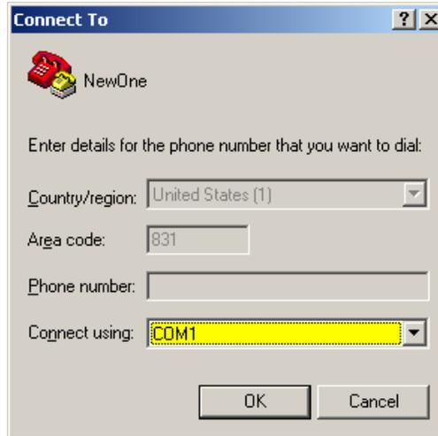
6. For "Connect using" select the COM port that the modem is on (do *not* select a modem driver), then select **OK**.
