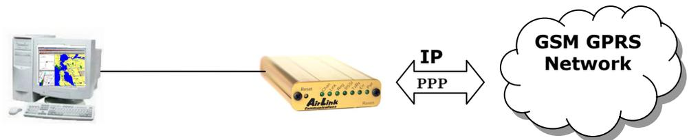
If the host establishes a PPP link to the Raven, a second PPP link is created between the Raven and the host. IP packets can then be sent to and received from the GPRS network.
