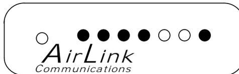
Note that the **RSSI** light may be flashing or solid, showing the strength of the signal. Also the **Tx/Rx** (transmit/receive) light will flash as data is transferred to and from the modem on the network.
