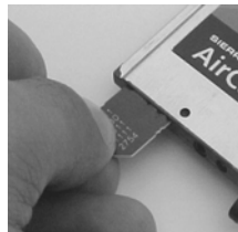
Figure 2-1: Inserting the SIM card into the AirCard SIM card slot
