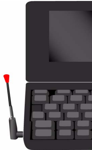
Figure 4-1: Proper positioning of the AirCard modem antenna for AirCard 850 modem / AirCard 860 modem
