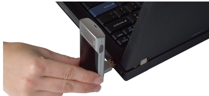
Figure 3-1: Correct way to insert the AirCard USB modem
