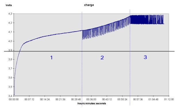
Figure 8: Li-Ion full charging waveform
