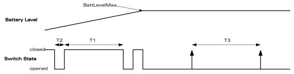
Figure 7: Ni-Cd / Ni-Mh charging waveform
