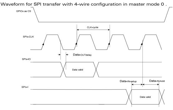
Figure 4: SPI Timing diagrams, Mode 0, Master, 4 wires
