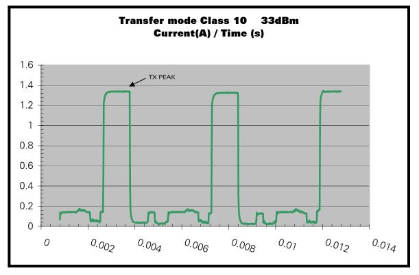
**3.2.2.4.4 Transfer Mode Class 10 Current Waveform**
