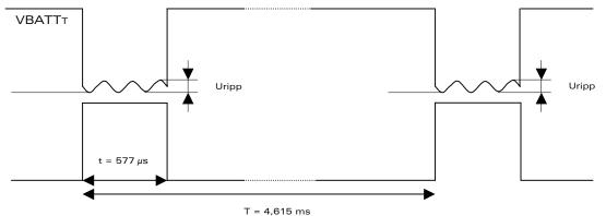
Figure 2: Power supply during burst emission
