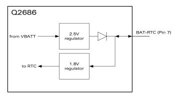
Figure 12: Real Time Clock power supply
