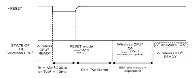
Figure 11: Reset sequence waveform
