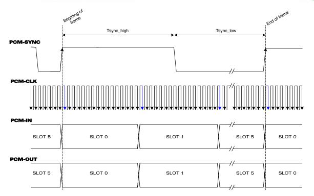
Figure 14: PCM frame waveform
