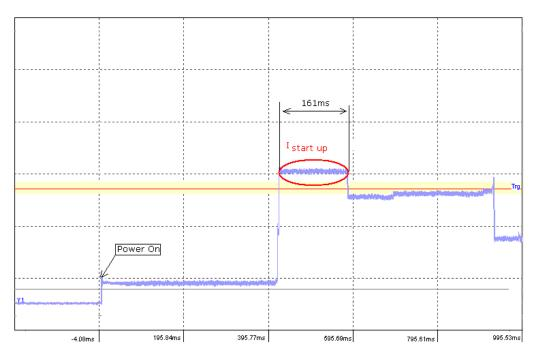
Figure 3: Start-up current waveform
