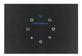
Short press Right button to move the cursor from 1 to 8, short press Left button to move the cursor from 8 to 1.
