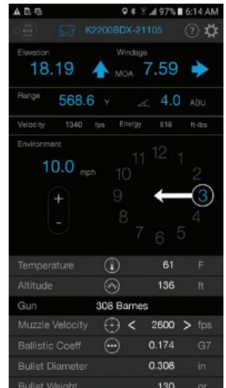
Angle modified range is the equivalent horizontal range to the target and is comparable to the “horizontal leg” of a triangle. AMR is also known as “rifleman’s rule” and uses the LOS range and angle of incline to calculate the horizontal distance the projectile travels between shooter and target. AMR is very accurate for shorter distances (i.e. < 400 yards) and archery.
