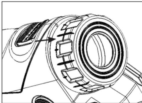
If you press the RANGE button while the rangefinder is off and continue to hold the RANGE button down, the rangefinder will automatically switch into SCAN mode within 1 second.
