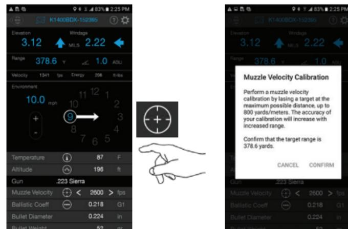
Use the MV Calibration routine at the farthest distance you intend to shoot. The greater the distance the more accurate the MV calculation will be. In this example the target was at 378 yards. Confirm your max target range.
