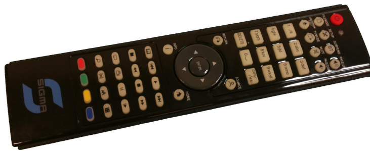
Figure 1 ZIRC Z-Wave / Infra-Red Remote Control
