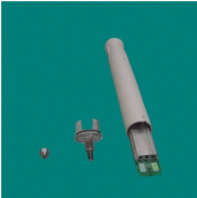
Smartpin mast with top cap removed and the electronics partially out
