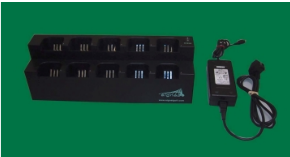
Pinpoint unit gang charger and power supply unit
