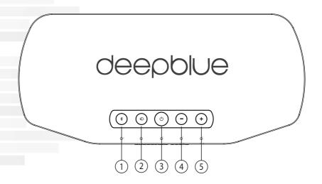
1 Bluetooth: Push and release to select the Bluetooth input. The blue LED will light for 10 seconds indicating the input is selected. Push and hold for several seconds to enter Bluetooth pairing mode. The Bluetooth LEDs will flash blue and white in this mode. Enter the Bluetooth menu on your device and select "deepblue2" to confirm the pairing. The Bluetooth LED will light solid blue and you will hear a double-beep when the deepblue² is connected to a Bluetooth device.
