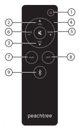
**Notes:** The first press of the BASS+ or BASS-buttons will display the current setting via the white LEDs. Subsequent presses within 10 seconds will adjust the bass setting. Each white LED represents 20% of the bass range. The lowest bass setting (1) is indicated by the left-most LED being lit 50%. The highest setting (10) is indicated by all the LEDs being fully lit.
