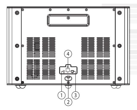
**AUX Analog Audio Input**: Accepts line-level analog input from a tuner, cassette deck, phono preamp or other type of line-level analog source.
