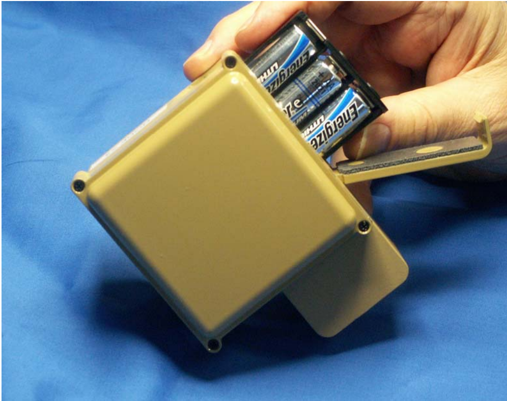
Figure 2 Inserting Battery Holder Into Node
