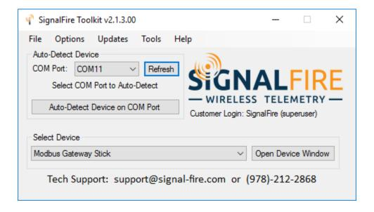
Select the COM port associated with the Flow Totalizer Node and click "Auto-Detect Device on COM Port." This will open the device configuration window, where all device settings can be configured.
