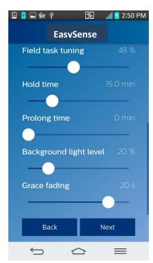
4. The App also provides an option to save this profile for future use by entering Profile name and Location. This profile will be saved. You can skip entering this information and program the EasySense sensor by press "Program EasySense".
