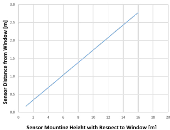
Figure 6 - Sensor horizontal distance from window vs. vertical sensor mounting height from window sill.
