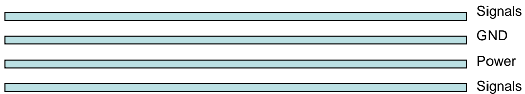
Figure 11: Typical 4-layer PCB construction
