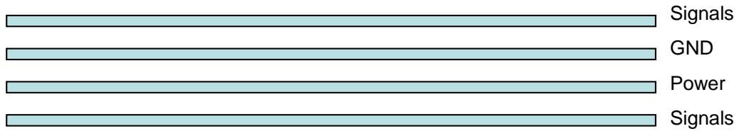
Figure 18: Typical 4-layer PCB construction
