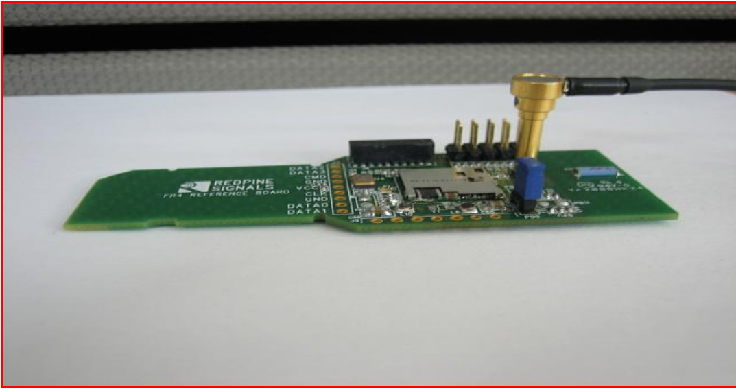
Figure 3: RF Cable Connected to the RS9110-N-11-02 Evaluation Board
