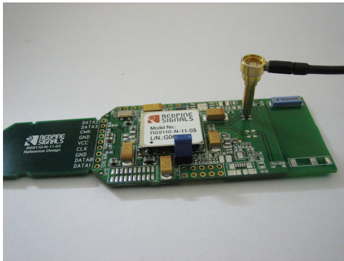
Figure 2: RF Cable Connected to the RS9110-N-11-03 Evaluation Board
