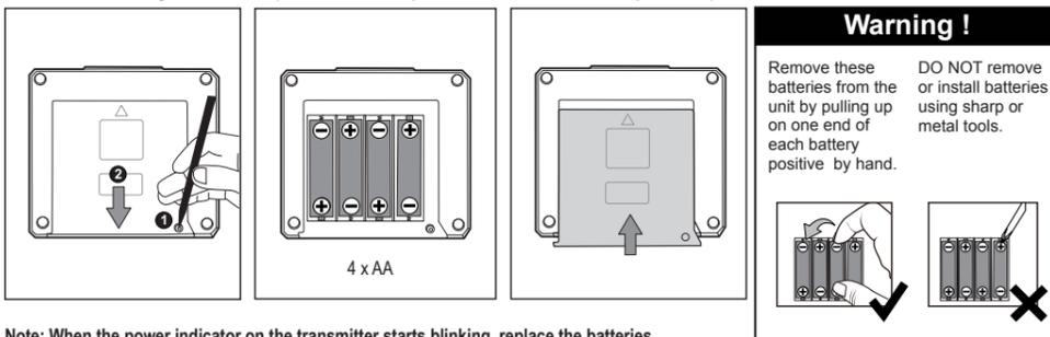
**Note: When the power indicator on the transmitter starts blinking, replace the batteries.**
