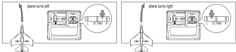
4. Push the direction stick toward left to turn the plane anticlockwise, and push the direction stick toward right to turn it clockwise. The plane turns depending on the speed difference between the left propellers and the right propellers.
