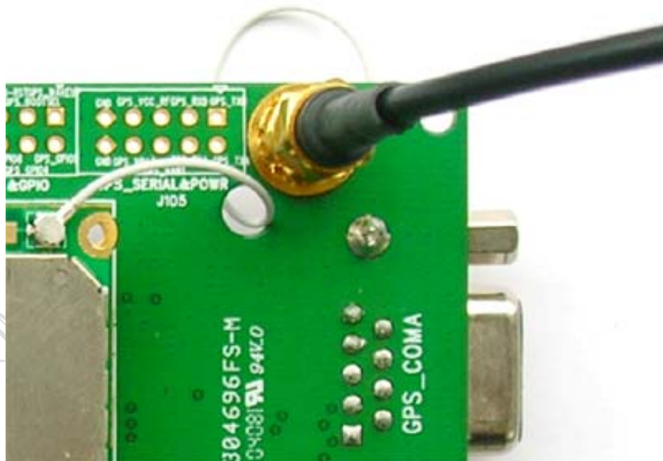
Figure 8: GPS antenna interface
