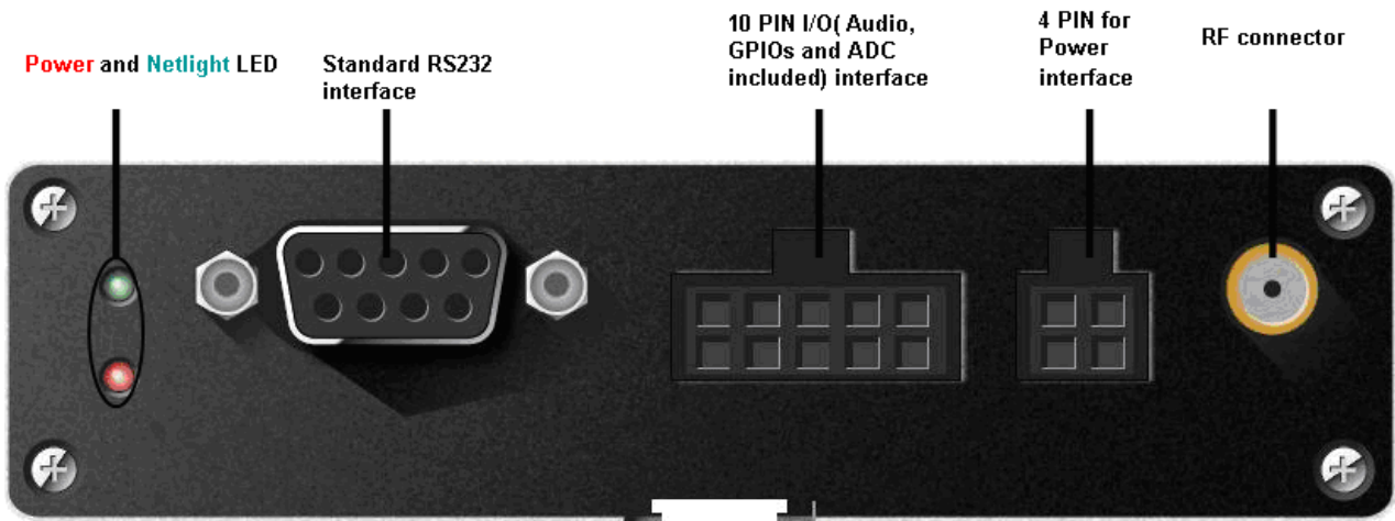
Figure 4: T5320+G interface Front view
