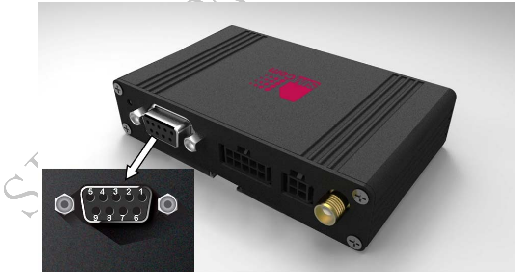
Figure 9: Pin assignment RS-232 (D-Sub 9-pole female)
