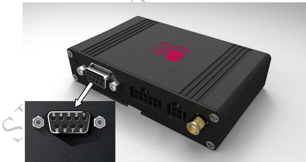
Figure 10: Pin assignment RS-232 (D-Sub 9-pole female)
