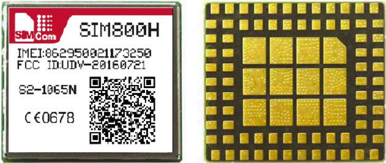
Figure 1: Top and Bottom view of SIM800H
