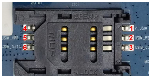
FIGURE 5: SIM card socket
