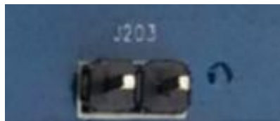
FIGURE 4: Power supply jumper
