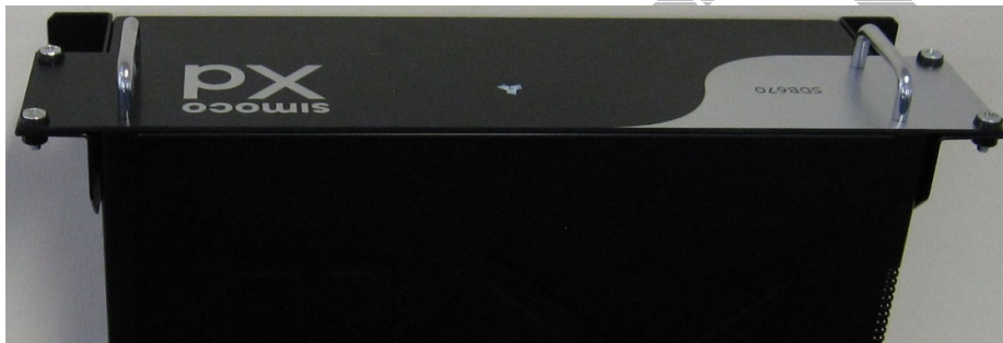
Figure 6. Base Station secured to Wall Mount.
