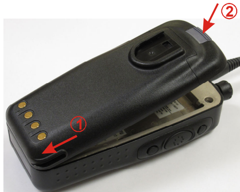
Figure 1. Fitting the Battery.
