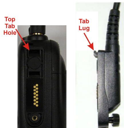
Figure 4. Fitting Audio Accessory/Programming Cable.
