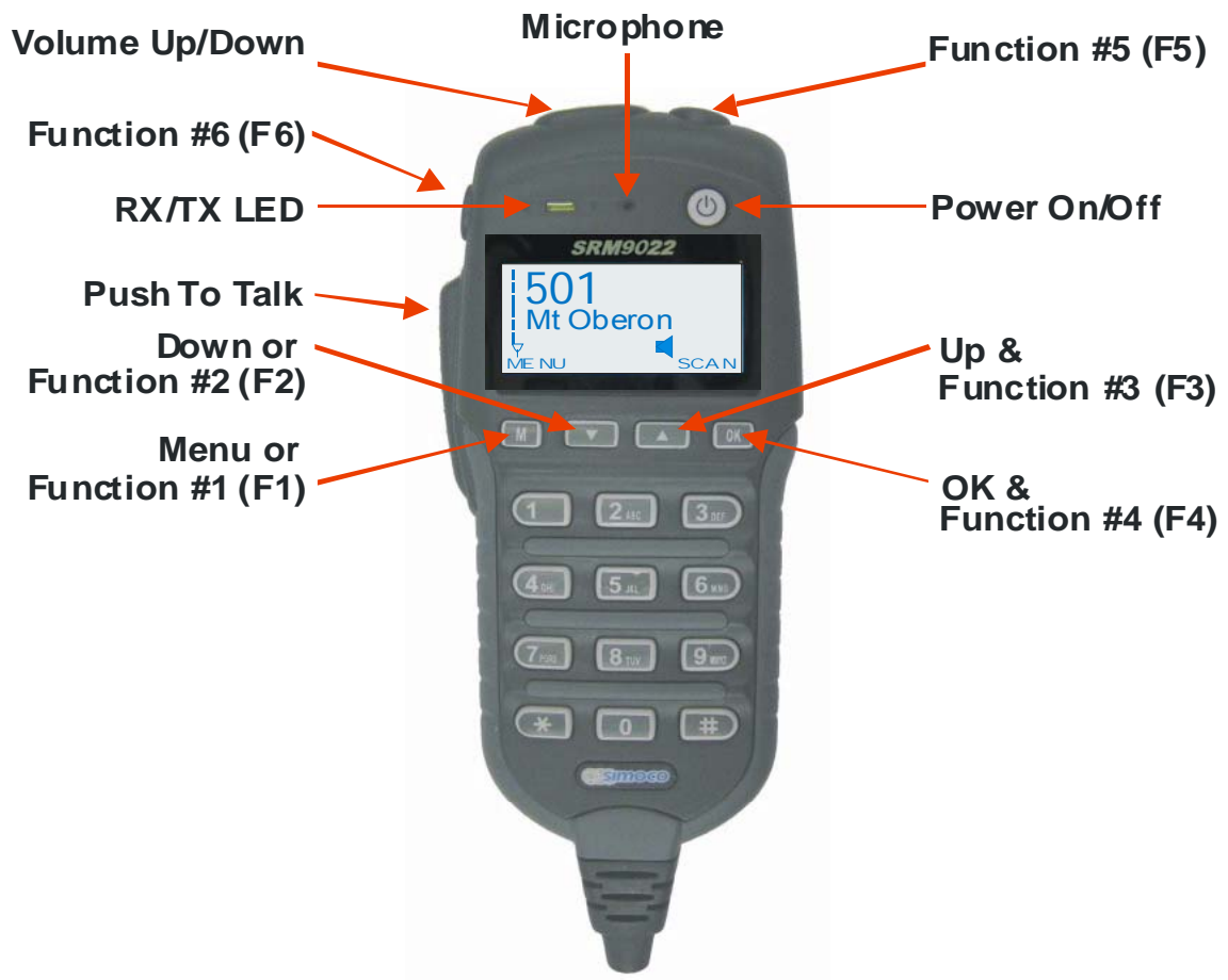
Figure 2-1 SRM9022 Controller Mic. Key Layout
