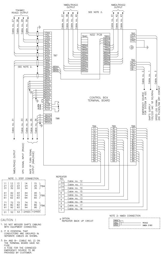
Figure 4-6 RGC12 External Wiring Diagram (N3-082093C)
