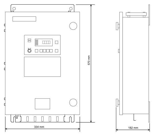
Figure 4-3 Control Box Dimensions
