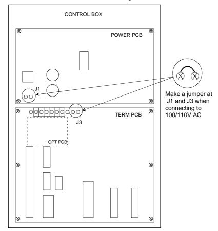
Figure 3-1 Jumper connection for 100/110V AC Mains supply
