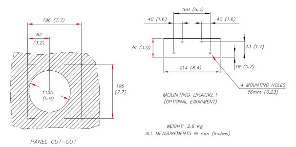
Figure 5-3 RSR68 Steering Repeater - Dimensions
