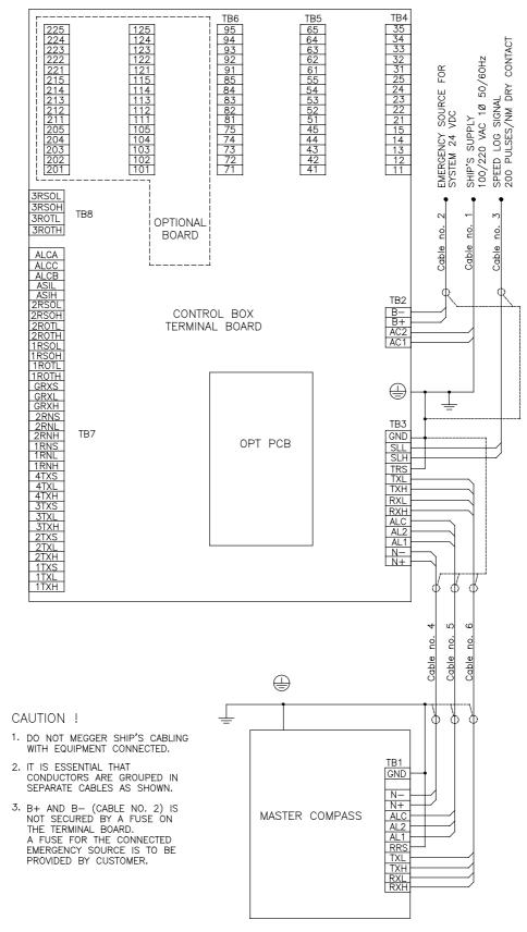
Figure 4-5 RGC12 Inter Unit Wiring Diagram (N3-082190)
