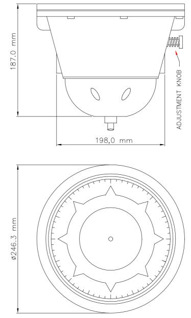
Figure 5-5 RP-41-1 Bearing Repeater - Dimensions (Drw. N4-710302A)
