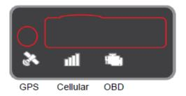
**OBD communication**: The OBD light change its status to solid on and comes 2 beeps with successful OBD communication.
