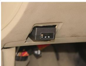
If the OBD port cover can not be closed back after device plugged in, please use OBD extension cable and mount the device in proper place.
