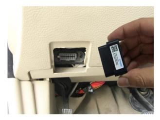
Start engine, with successful OBD communication the OBD light changes its status to solid on. Then device begins to connect app, with successful network registration the Bluetooth light change its status to blinking every 2 times.
