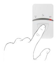
**Power button:** To power on/off the tracker. Long press it until red LED turns on, tracker is powered on; Long press it until all LED turns off, tracker is powered off.
