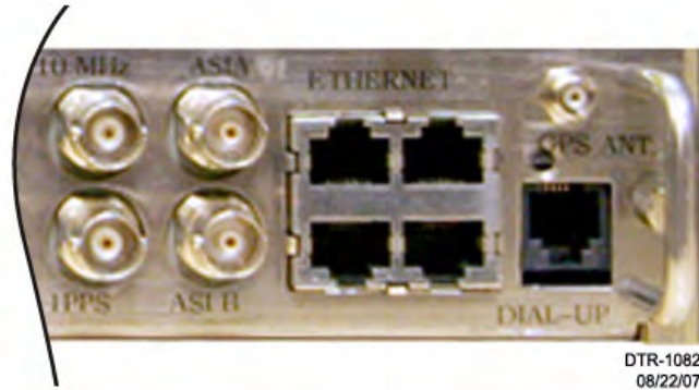
Figure 4-4 Ethernet Ports on Main Controller Back Panel
