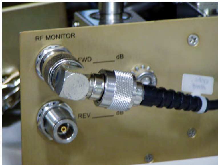
Figure 4-3 RF Monitor Connectors on Junction Box Panel
