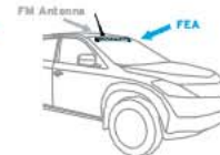
FRONT ROOF TOP MOUNTED FM ANTENNA
