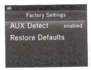
If you are using the older model Vehicle Dock from the Universal Xpress Car Kit, and plan to use *Power*Connect or FMDA as the audio connection option, you will need to disable AUX Detect. Please read the additional instructions, "Using the Vehicle Dock From the Universal Xpress Car Kit" on page 88. Once AUX Detect is disabled, you'll have to turn the FM Transmitter On. Refer to "Turn FM Transmitter On/Off" on page 89.
