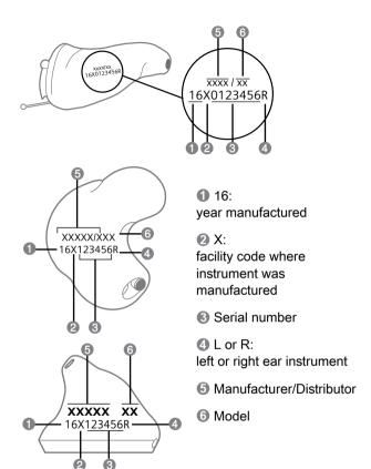
For BTE and RIC instruments, the year of manufacture is derived from the second digit:
