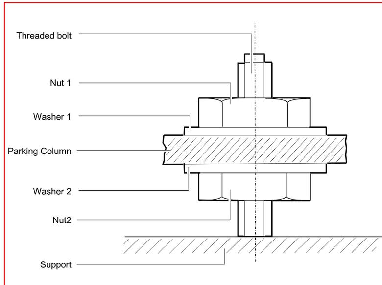
All three No. 2 washers must be absolutely level (use a spirit level if necessary).
