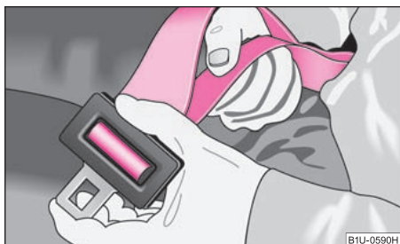
Fig. 121 Extending the pelvic belt
