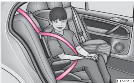
Fig. 135 Child seat in Group 2 installed on the rear seat facing the direction of travel
