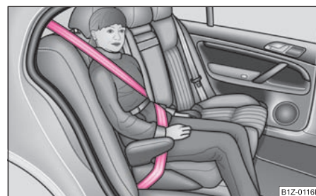
Fig. 136 Child seat in Group 3 installed on the rear seat facing the direction of travel
