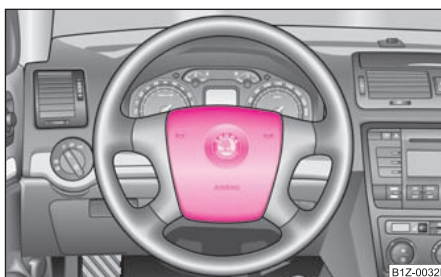
Fig. 122 Driver airbag in the steering wheel
