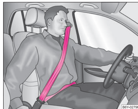
Fig. 116 Routing of webbing over the shoulders and the lap belt
