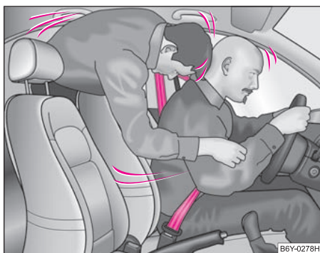
Fig. 115 The rear seat occupant is thrown forward if not wearing a belt
