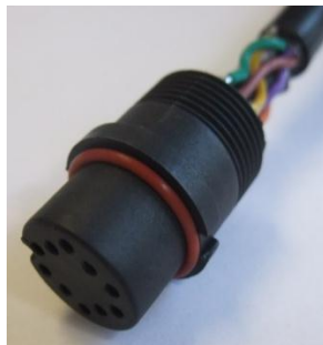
Figure 36 O-Ring over Connector Body
