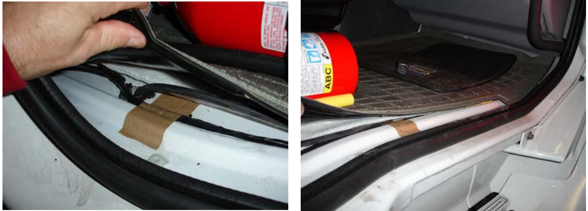
Figure 22 Sample Cable Placement in a Vehicle Cab
