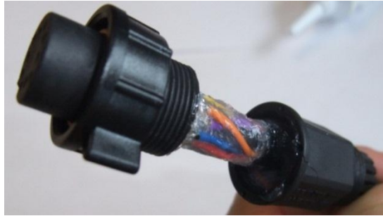
Figure 38 Silicone in the Grommet
