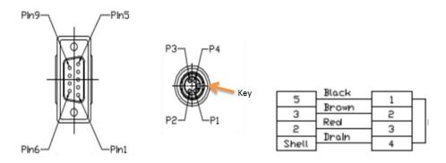
This interface can be used by an operator only to control, configure, and troubleshoot IBR, but not for general network connectivity or data transmission. Pin-outs of the four-pin serial connector are shown in the table below.
