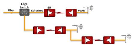
NOTE: The installer is responsible for ensuring that the system is used exclusively for fixed, point-to-point operations.
