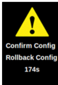
Figure 74 - Icon Displayed When Rollback Is Enabled and a Critical Change Is Made on the GUI, showing timer countdown
