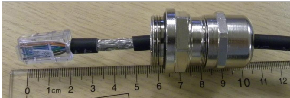
Figure 19 - Expose the cable screen starting at 35mm distance, and running up to 50mm from end of plug
