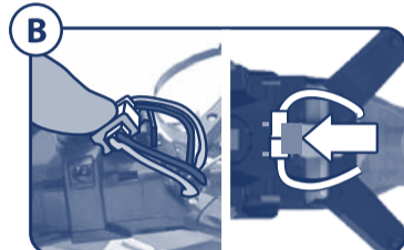
Align forward facing edge of connectors against short tabs before snapping into locked position against connector's tab.
