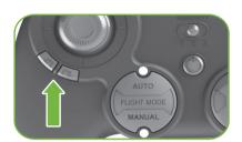
IF THE DRONE SPINS COUNTER-CLOCK-WISE (VIEWED FROM ABOVE): Press the 🔼 button several times until the drone stops spinning.
