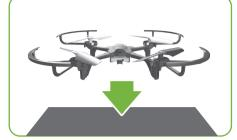
Place the drone on level surface for calibration.
